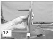
Slide the mount shaft onto the channel. Tape a second channel into it with half of it above the shaft. (this second shaft is to help in alignment)
