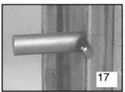
Tack weld the shaft in place.
