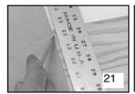
The 1/4" extra compensates for the felt channel.
