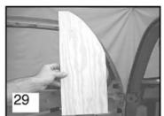
Here we have cut out a piece of wood to aid in the positioning of the bottom front mount brackets.
