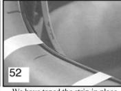
We have taped the strip in place and are ready to drill the pilot holes.
