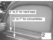
Trace the window opening on to a poster board. Leave the board long at the bottom and be precise.
