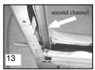
Slide assembly through hole. The channel sticking up represent the glass position.
