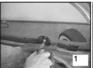
Remove all hardware. Cut away any metal that will interfere with the one piece glass.
