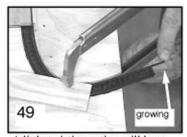
A little twisting action will keep the inside bead of the whisker from binding and buckling while you form it.
