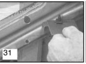
With the channel in position determine where to place the bottom mount brackets. Position and weld accordingly.
