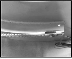
5) Make sure the back side has proper clearance for the electronics. Check both sides, there is a small resistor on the under side of this LED strip. (NOTE: not all LED strips have these components. This may or may not be necessary for you.)
