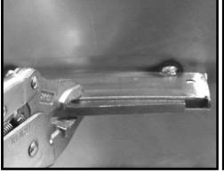
8) The steel plug will help keep everything in alignment and work as a heat sink to minimize distortion.
