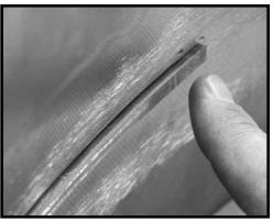
10) Dress the welded area and prepare 11) A small amount of body filler will be it for the lens. Pre fit the lens. Bolt it in place then begin sanding it down. Use 50 grit to cut it down within an 1/8". Then use finer abrasives.
