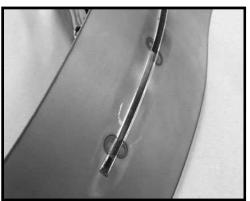
Spot weld the housing into place with the 1/8" protruding. Always have the steel welding plug clamped in place.
