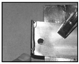
4) Weld ends. Use a 1/4" steel welding plate spacer or make a stack of steel plates that equal the thickness of the lens.
