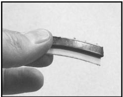
13) Final assembly: Bolt lens in place. 14) You kit comes with a small strip of black sticky putty. Use this to seal the ends of the U channel.
