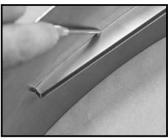
2) Assemble lens and steel plates and slip it into the slot. Position the assembly and mark where to trim. Make sure the bolt holes are accessible.
