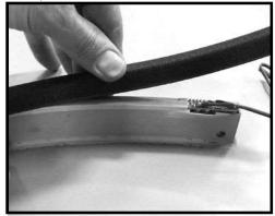
Lay LED strip into slot. And tape down with 3/4" tape. Trim rubber U channel to length and press over LED.
