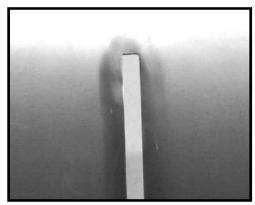
1) Mark and cut out slot for LED assembly. Make a clean cut to minimize the weld process.
