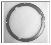
**STEP TWO:** LAMP ASSEMBLIES This is how the lamp base sets in the bucket. Notice the three large round holes will line up with the mount tabs. Notches align the lamp.
