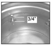
Install the lamp base. Screw them down until you have a 3/4" measurement from the mount tab to the lamp base.
