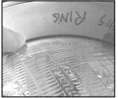
Snap the trim ring in place and check the gap between the lamp and ring. Adjust the lamp until you have a nice clean gap. Now you can fine tune to aim the lamps.
