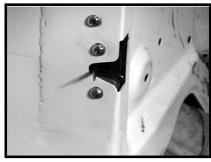
5) Mark the position for the striker. To do so stick your scribe through the latch as shown and mark the jamb with the door closed.
