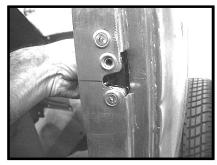
4) Here the plate has been welded in and dressed with a grinder. Now bolt the latch into place.
