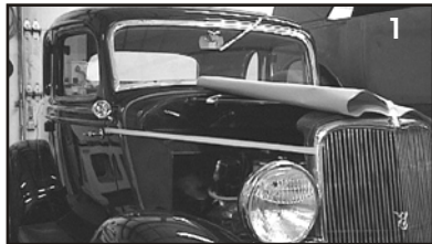
1 With the grill positioned run tape along the bottom of the belt line of the cowl to the grill. Note: the top of the tape represents the bottom of the hood.
