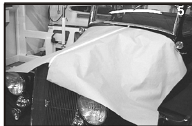
5 YOU MUST start at the center and work your way to the sides. Pull paper tight and anchor it down the center.
