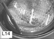
REMOVE THE SCREWS AND INSTALL THE LAMPS. INSTALL THE LAMP RETAINER RING.
