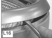
ASSIST THE SECOND AND THIRD WITH A BLUNT INSTRUMENT. CHECK THE GAPS AND MAKE ANY NECES-SARY ADJUSTMENT BEFORE PAINT-ING
