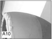
HERE YOU CAN SEE HOW THE FILLER WAS APPLIED. REMOVE THE TAPE JUST AS THE FILLER BEGINS TO HARDEN. REMOVE THE TRIM RING AND THE CAULKING.
