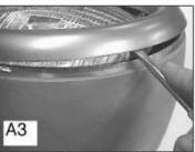
TO INSTALL THE TRIM, SLIP THE TOP CLIP IN PLACE AND ASSIST THE SEC-OND AND THIRD CLIP WITH A BLUNT INSTRUMENT, TRIM RING MAY TEND TO SEE-SAW BUT SHOULD BE SNUG NOTE: ON FINAL ASSEMBLY IT IS BEST TO PUT TWO LAYERS OF MASKING TAPE ON THE PAINTED EDGE SO YOU DO NOT SCRATCH THE PAINT!
